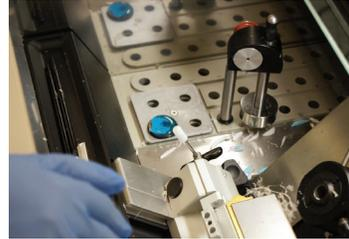
A base of blue polyvinyl gel holds tissue samples. Both are placed on the black dial at the right, and a blade slices layers of tissue for microscope slides.
